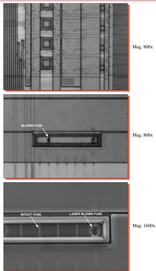
Figure 24. Optical and SEM views of typical fuses.
