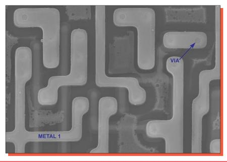
Figure 15. Topological SEM views of metal 1 patterning. Mag. 6500x, 0°.
