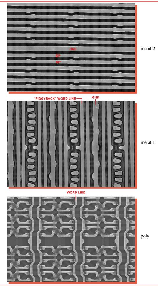
Figure 30. Topological SEM views of the SRAM cell array. Mag. 3200x, 0°.
