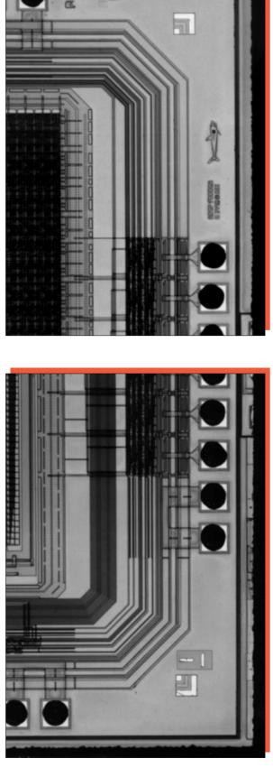
Figure 5. Optical views of die corners. Mag. 80x.
