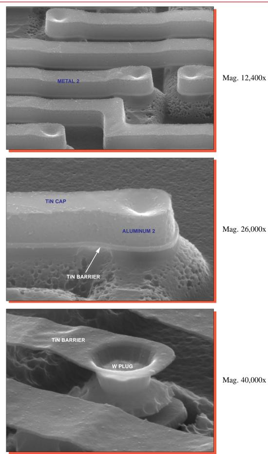
Figure 12. Perspective SEM views of metal 2 step coverage, barrier, and plug. 60°.
