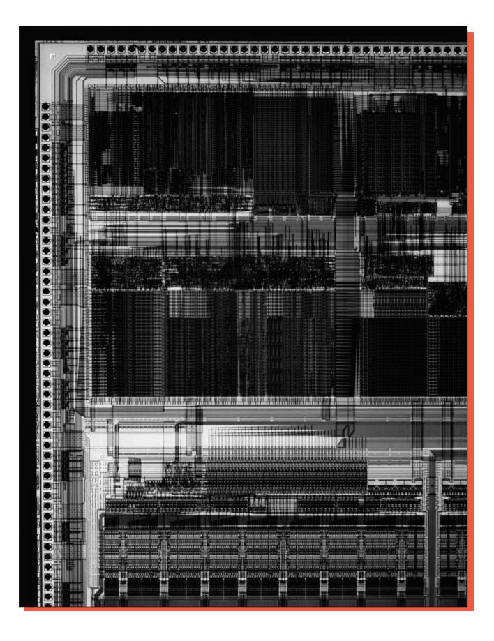
Figure 3. Portion of the Analog Devices ADSP-21062-KS-160 die. Mag. 26x.
