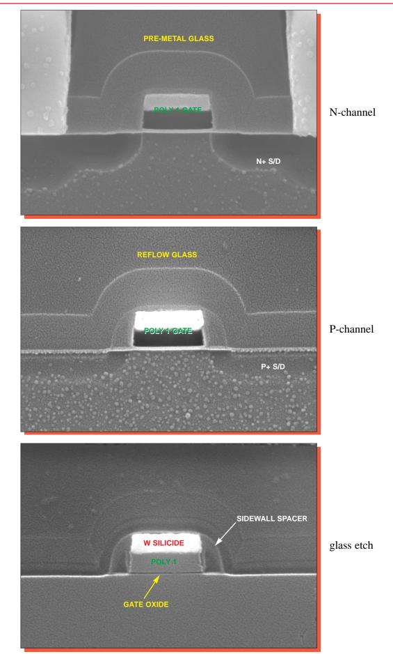
Figure 21. SEM section views of typical transistors. Mag. 52,000x.
