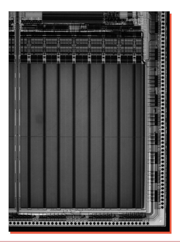
Figure 3c. Remaining portion of the Analog Devices ADSP-21062-KS-160 die. Mag. 26x.
