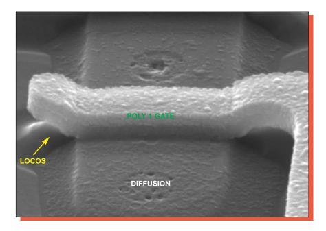
Figure 20. Perspective SEM views of poly 1 coverage. 60°.
