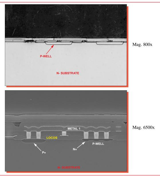
Figure 23. Section views illustrating well structure.
