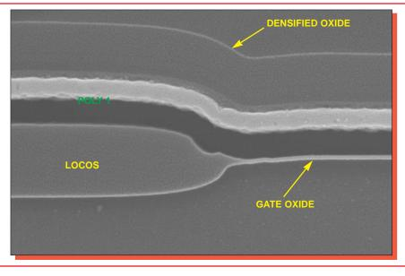
Figure 22. SEM section view of typical birdsbeak. Mag. 52,000x.
