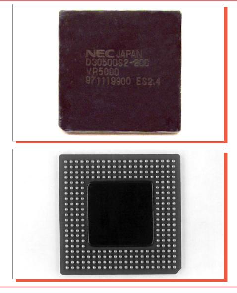
Figure 1. Package photographs of the NEC 79VR5000 RISC. Mag. 2x.
