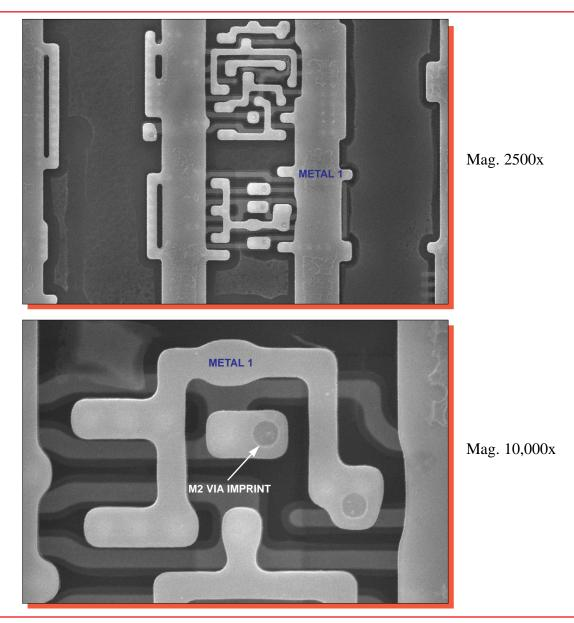
Figure 21a. Topological SEM views of metal 1 patterning.  $0^{\circ}$ .
