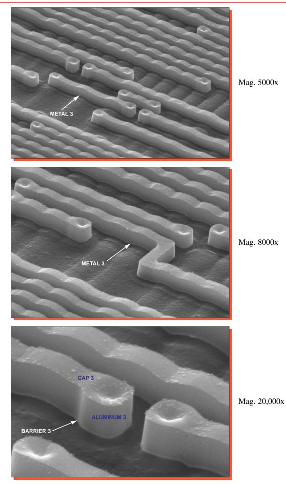
Figure 15. Perspective SEM views of metal 3 integrity.  $60^{\circ}$ .
