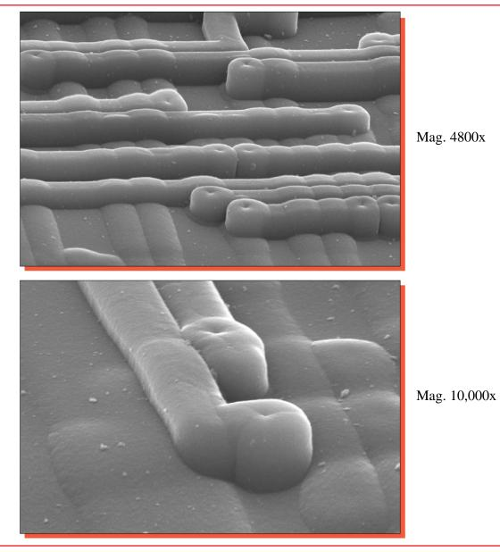
Figure 11. SEM views of passivation coverage. 60°.
