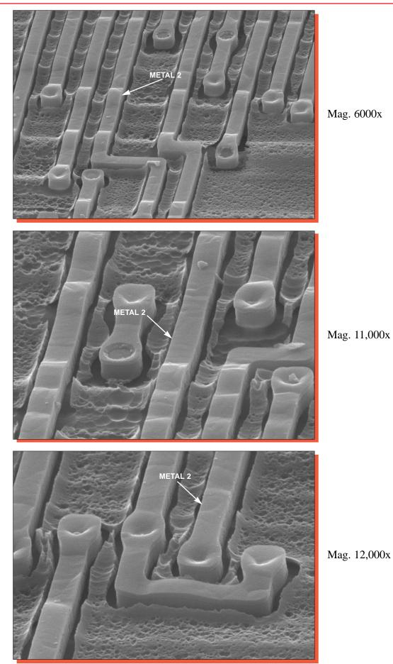
Figure 19. Perspective SEM views of metal 2 integrity. 60°.
