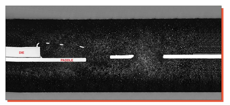
Figure 4a. Optical views of the PLX Technology package illustrating general construction. Mag. 20x.
