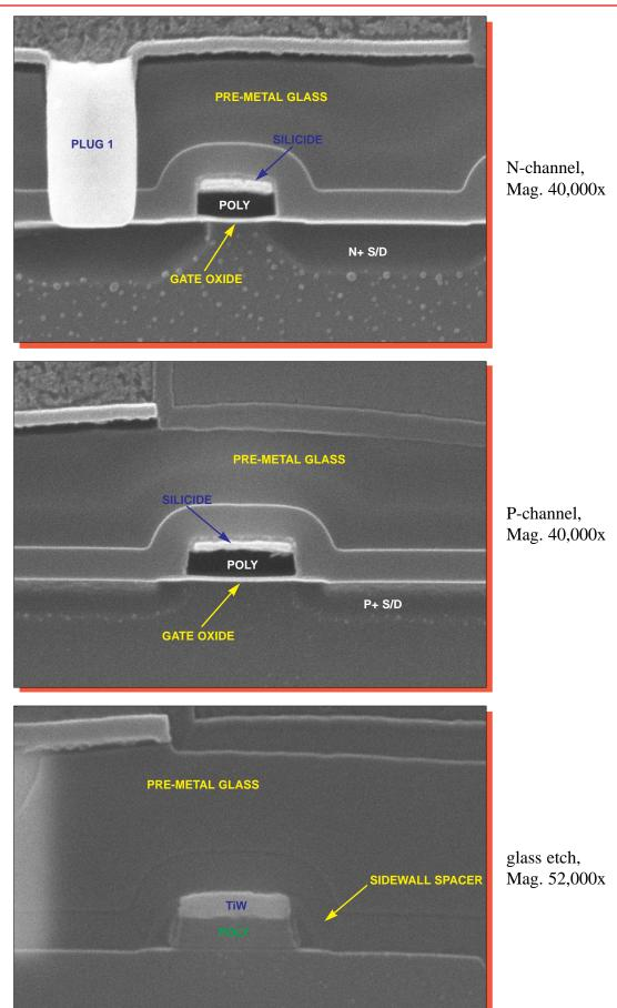
Figure 26. SEM section views of typical transistors.
