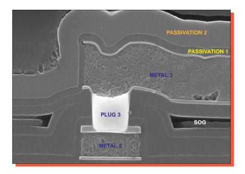
Figure 16. SEM section views of metal 3-to-metal 2 vias.
