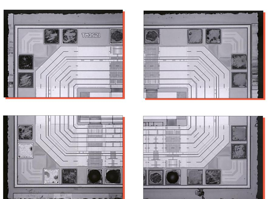
Figure 9a. Optical views of the die corners on the PLX Technology PCI9080 device. Mag. 160x.
