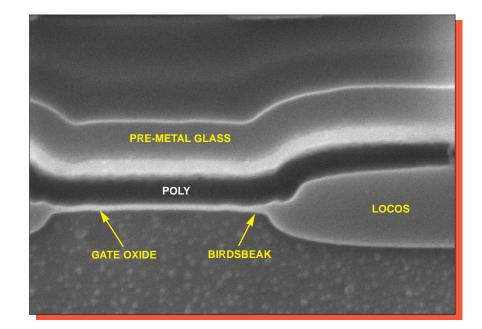
Figure 27. SEM section view of a local oxide birdsbeak. Mag. 52,000x.
