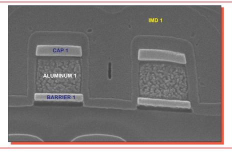
Figure 21. SEM section view of metal 1 line profiles. Mag. 40,000x.
