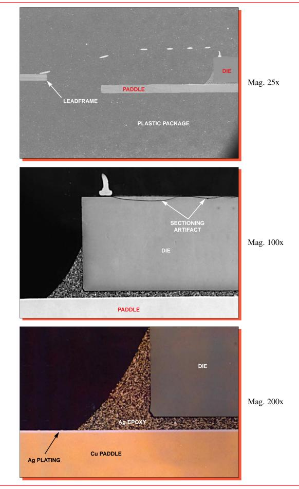
Figure 6. Optical views of dicing and die attach.
