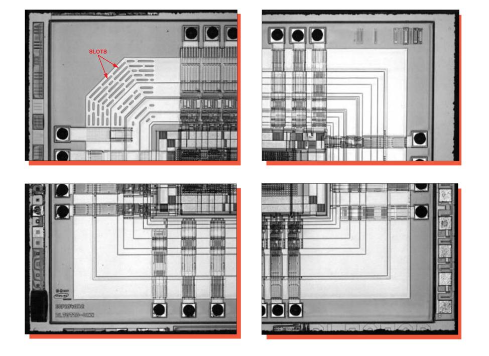
Figure 10. Optical views of die corners. Mag. 100x.
