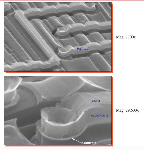
Figure 18. Perspective SEM views of metal 2 integrity. 60°.
