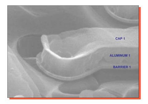
Figure 21. Perspective SEM views of metal 1 integrity.  $60^{\circ}$ .
