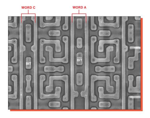
Figure 29. Topological SEM views of SRAM cell. Mag. 2400x, 0°.
