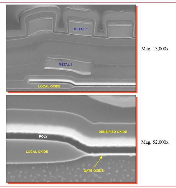
Figure 27. SEM section views of a typical birdsbeak.
