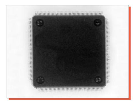
Figure 1. The QLogic ISP1040B package. Mag. 2.5x.
