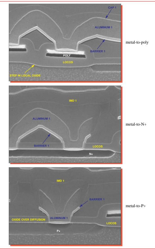
Figure 22. SEM section views of typical contacts. Mag. 26,000x.
