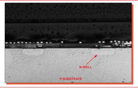
Figure 26. Optical view of well structure. Mag. 1240x.
