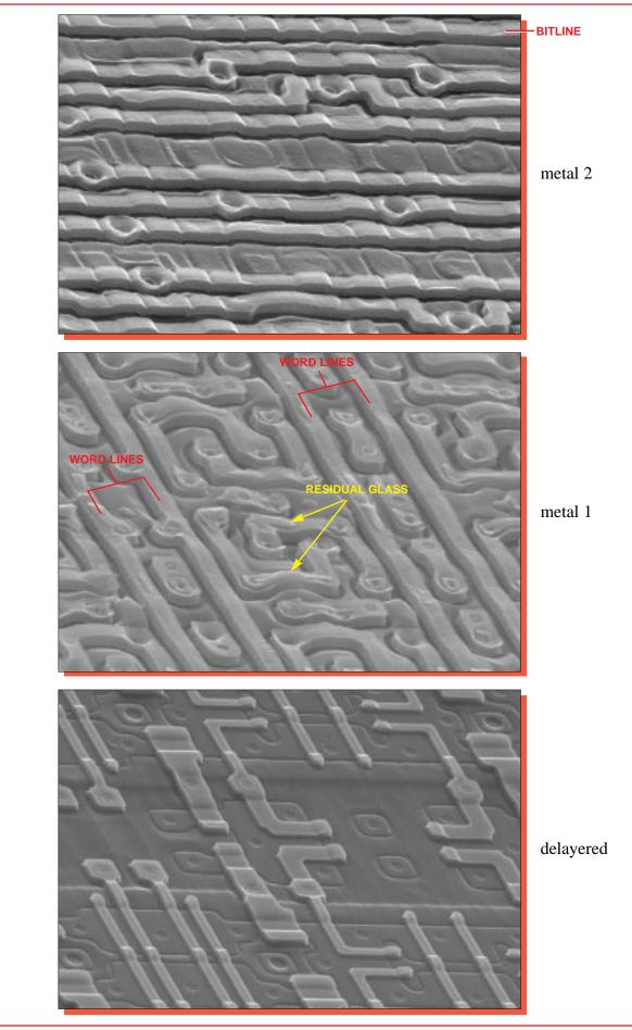
Figure 28. Perspective SEM views of the SRAM cell array. Mag. 4200x, 60°.
