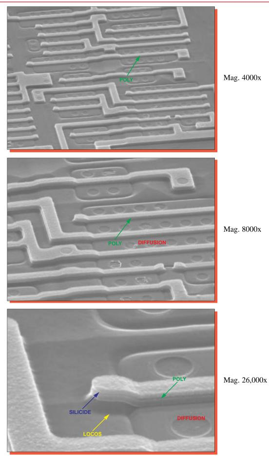
Figure 24. SEM views of polycide coverage.  $60^{\circ}$ .
