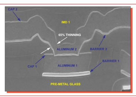
Figure 18a. SEM section view of a metal 2-to-metal 1 via. Mag. 26,000x
