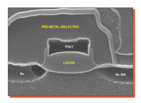
Figure 32. SEM section views of programmed cells. Mag. 52,000x.
