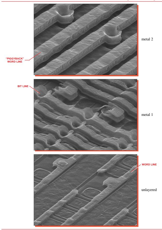
Figure 27. Detailed perspective SEM views of the MROM array. Mag. 10,000x, 60°.
