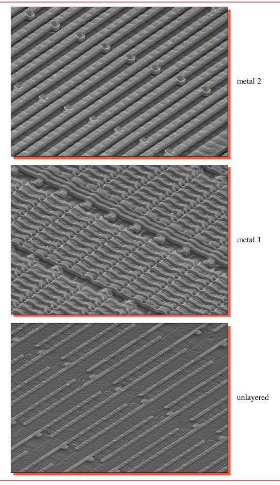
Figure 26. Perspective SEM views of the MROM array. Mag. 2500x,  $60^{\circ}$ .
