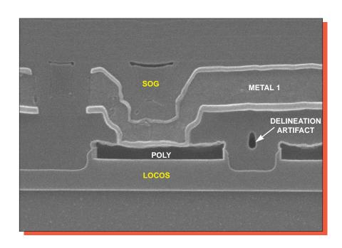
Figure 17. SEM section views of typical metal 1 contacts. Mag. 26,000x.
