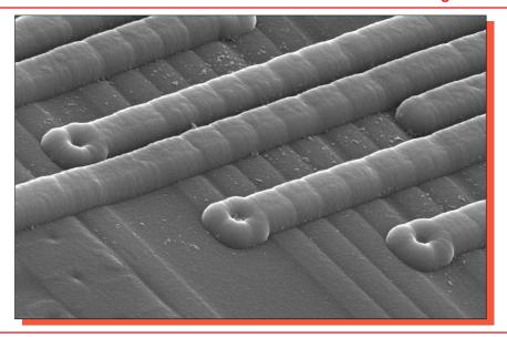
Figure 9. SEM view illustrating final passivation. Mag. 4800x, 60°.
