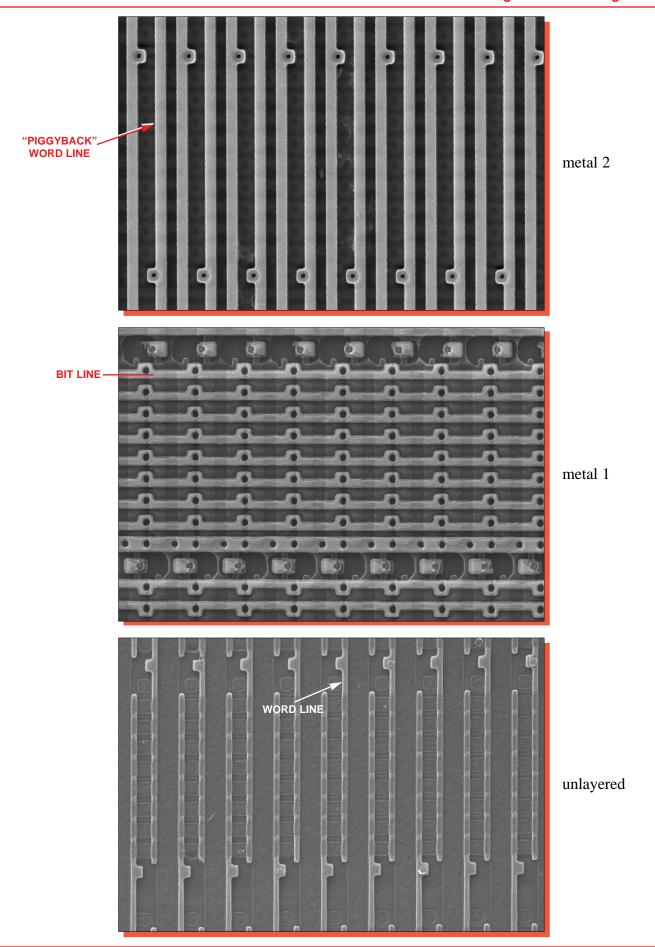
Figure 29. Topological SEM views of the MROM array. Mag. 2100x, 0°.
