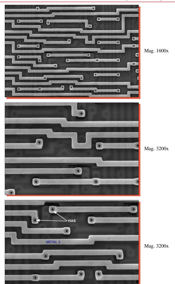
Figure 11. Topological SEM views of metal 2 patterning.  $0^{\circ}$ .
