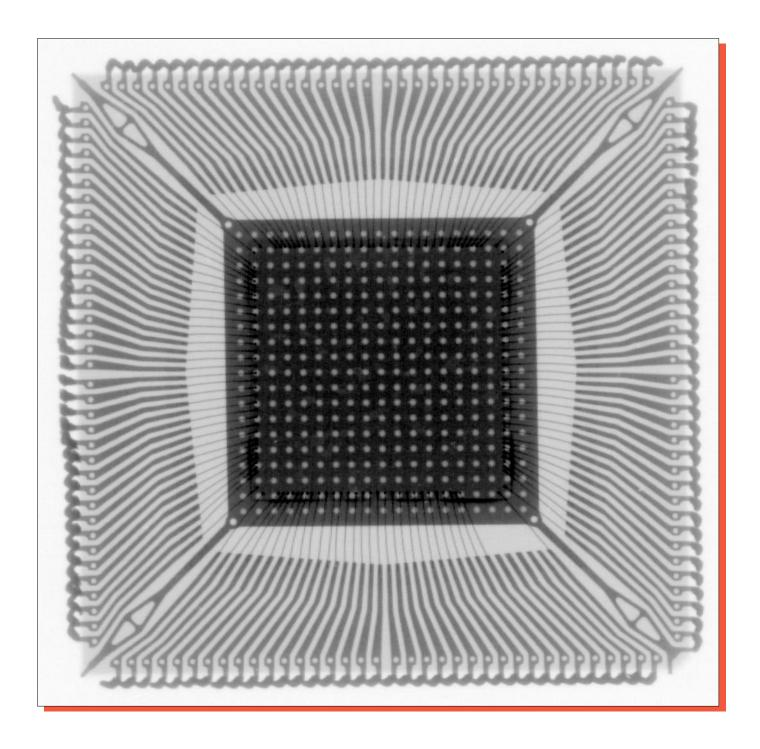
Figure 2. X-ray of the Rockwell 11577-11. Mag. 8x.
