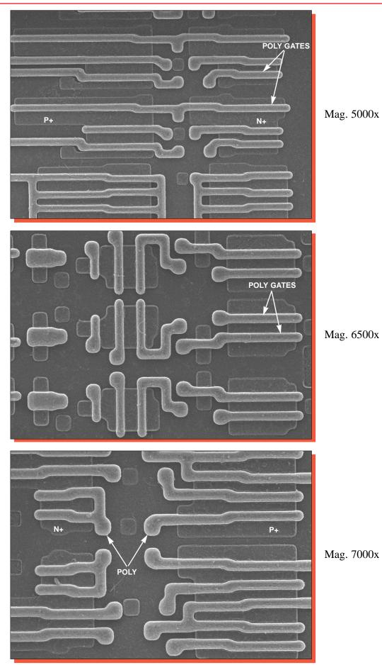
Figure 34. Topological SEM view of poly patterning. 0°.
