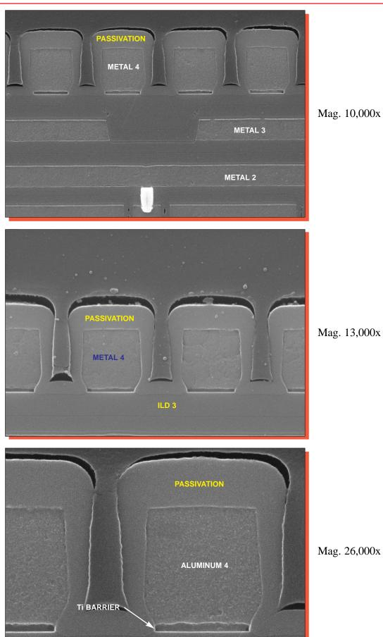
Figure 15. SEM section views of metal 4 line profiles.
