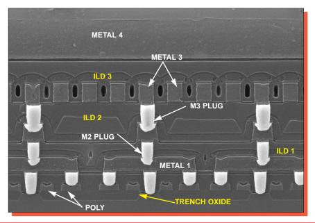
Figure 13. Glass etch section views illustrating general structure. Mag. 9000x.
