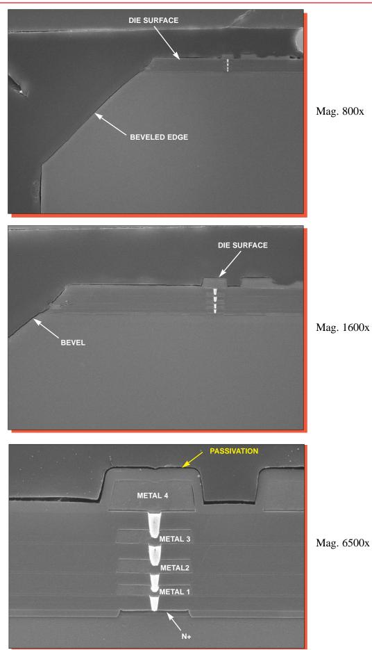
Figure 8. SEM section views of the edge seal structure.
