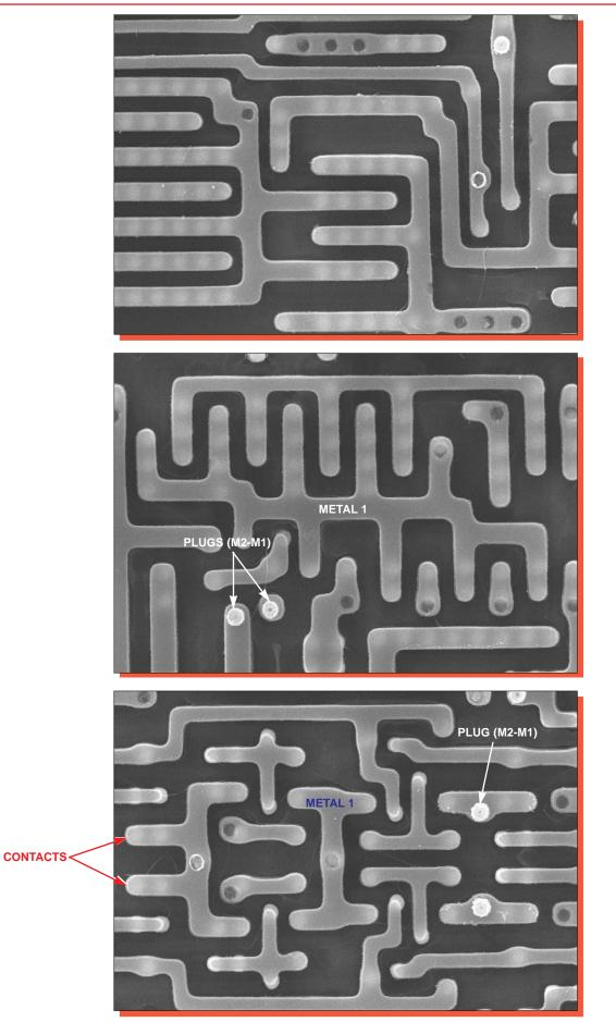
Figure 30. Topological SEM views of metal 1 patterning. Mag. 7000x, 0°.
