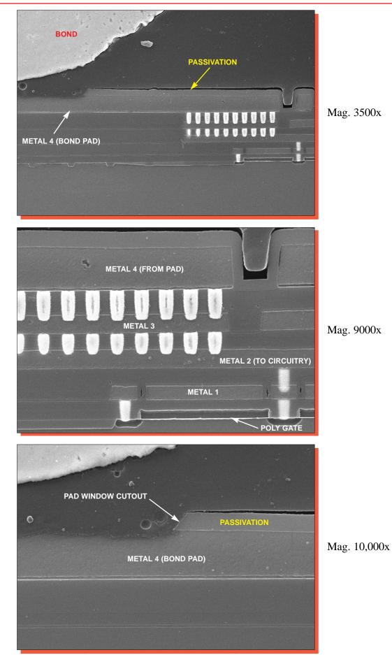
Figure 5. SEM section views of the pad structure.
