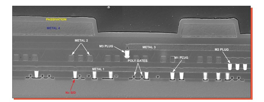
Figure 12. SEM section view illustrating general device structure. Mag. 6500x.
