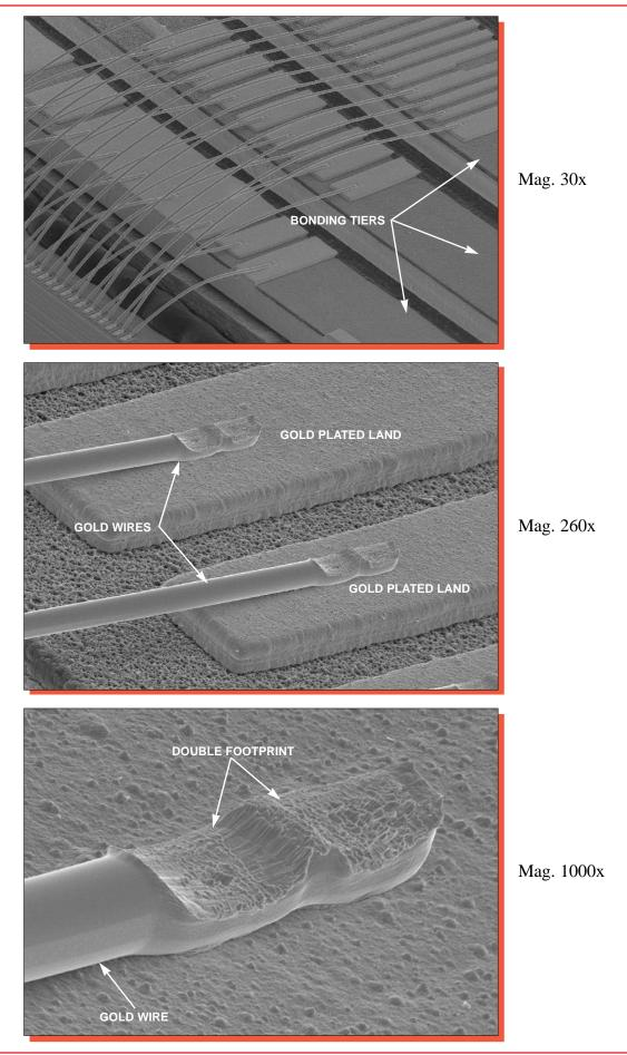
Figure 3. SEM views of typical wirebonding.  $60^{\circ}$ .
