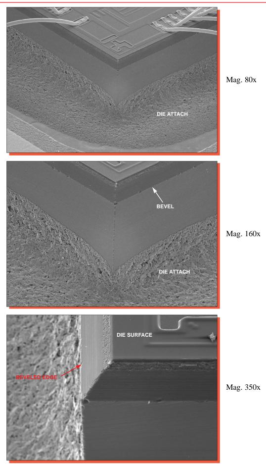
Figure 7. SEM views of a die corner illustrating dicing and die attach. 60°.
