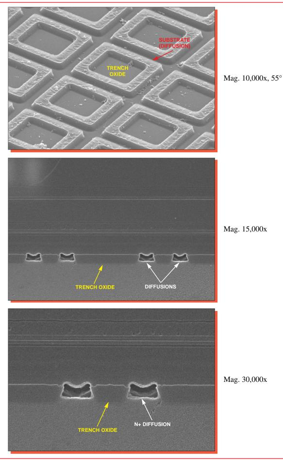
Figure 39. SEM views illustrating anti-dishing patterns.
