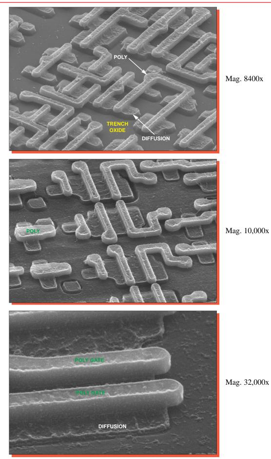
Figure 35. Perspective SEM views of poly coverage.  $55^{\circ}$ .
