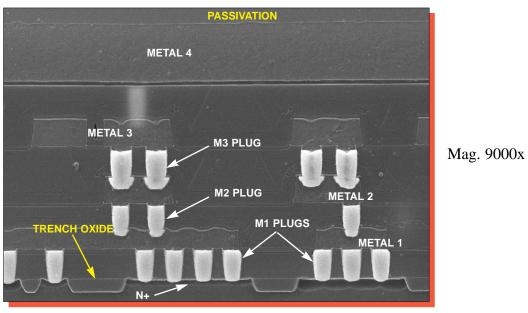
Figure 12a. SEM section views illustrating general device structure.
