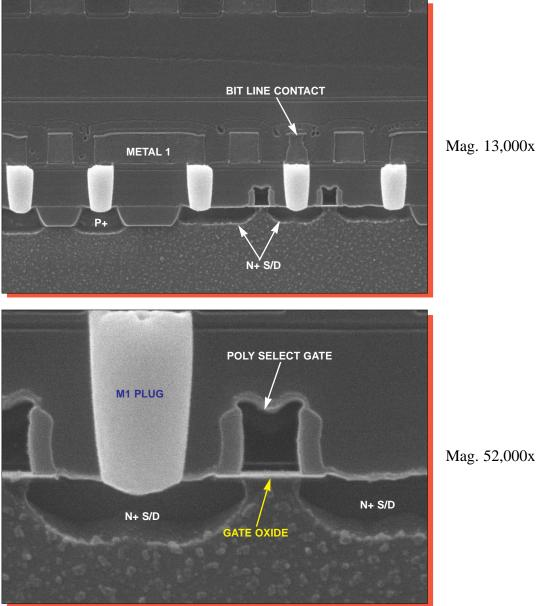
Figure 47. SEM section views of a Cache SRAM cell (perpendicular to word lines).
