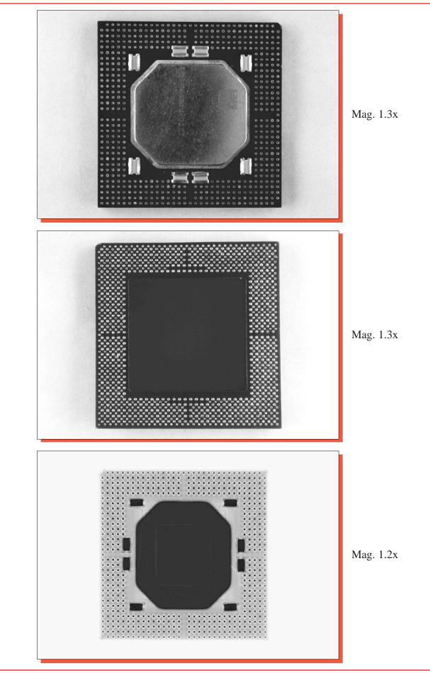
Figure 1. Package photographs and x-ray view of the Intel Pentium II Processor.
