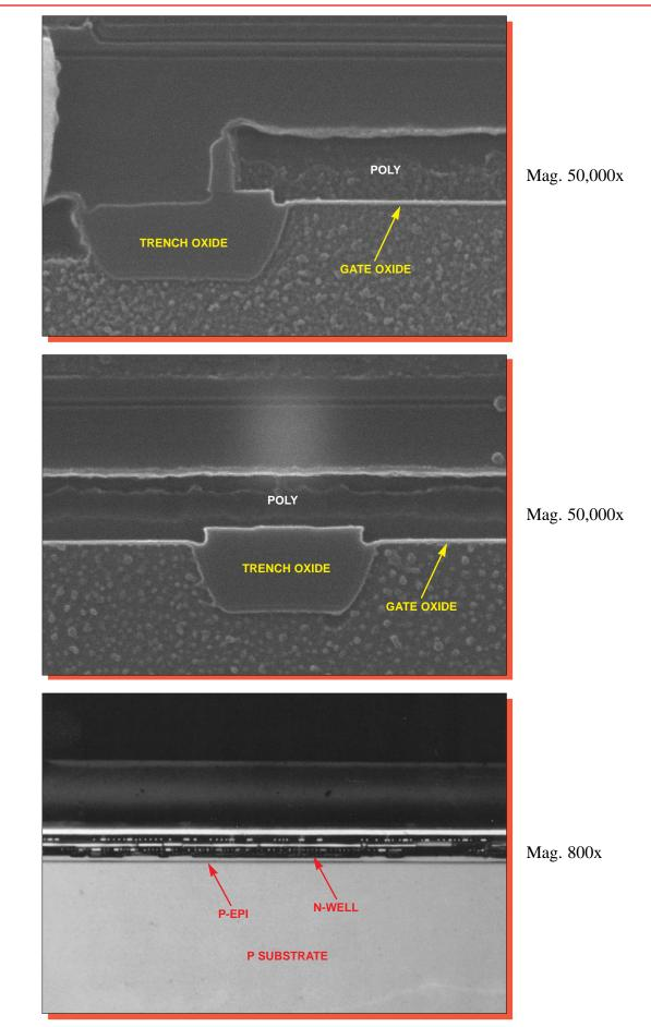
Figure 40. Section views illustrating trench oxide and well structure.
