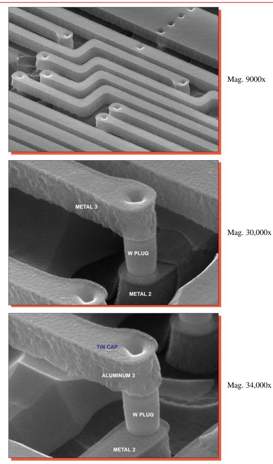
Figure 22. SEM views of metal 3 coverage. 55°.
