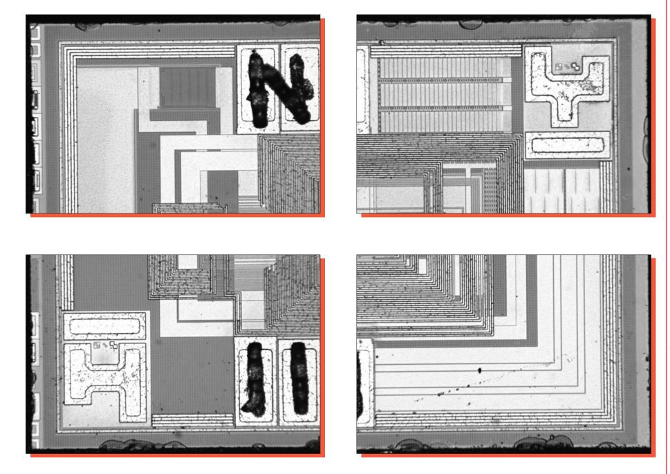
Figure 11. Optical views of die corners. Mag. 225x.
