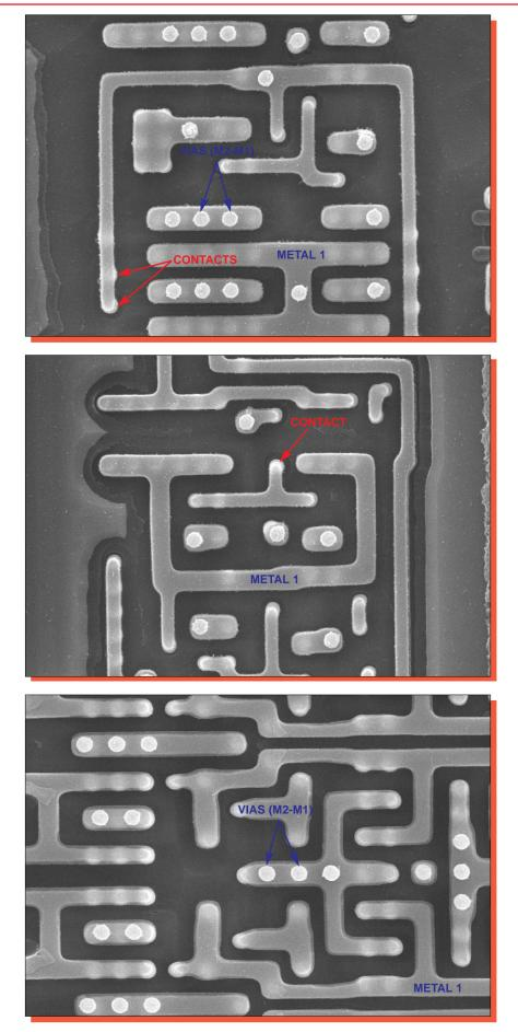
Figure 26. Topological SEM views of metal 1 patterning. Mag. 6500x,  $0^{\circ}$ .
