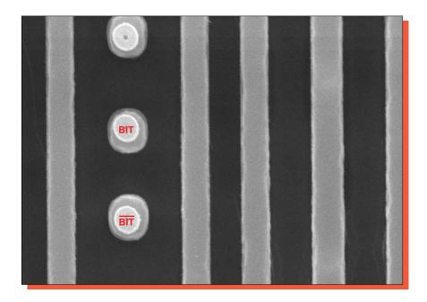
Figure 44. Topological SEM views of a Cache SRAM cell. Mag. 13,000x, 0°.
