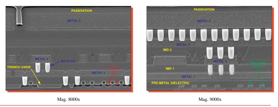
Figure 9. SEM section views illustrating general device structure.
