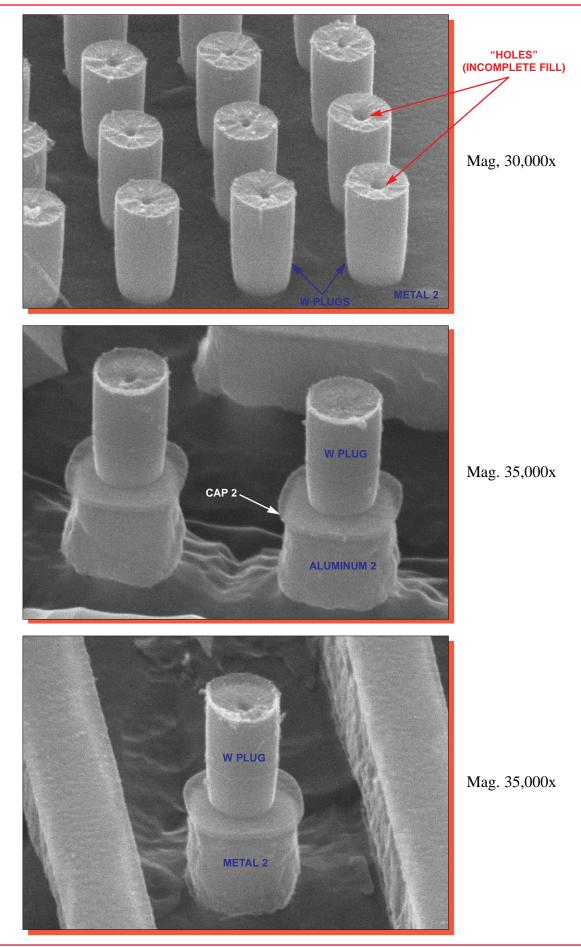
Figure 18. SEM views of metal 3 tungsten plugs.  $55^{\circ}$ .
