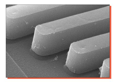
Figure 11. SEM views of metal 4 patterning and coverage.
