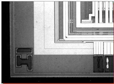
Figure 5. Optical views of the die corners. Mag. 100x
