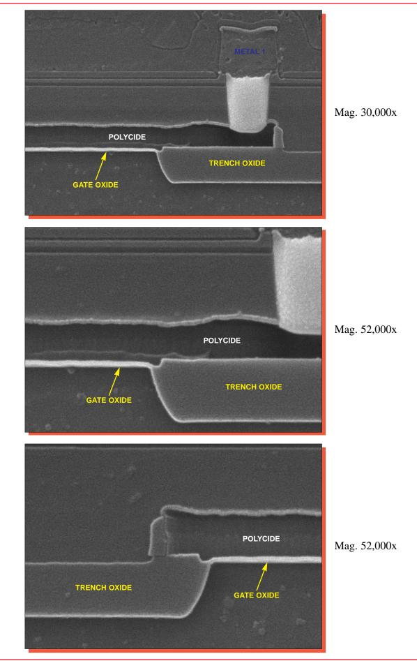
Figure 38. SEM section views of trench oxide isolation.
