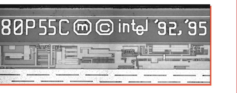
Figure 4. Die identification markings. Mag. 200x.
