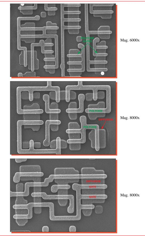
Figure 34. Topological SEM views of polycide gates.  $0^{\circ}$ .
