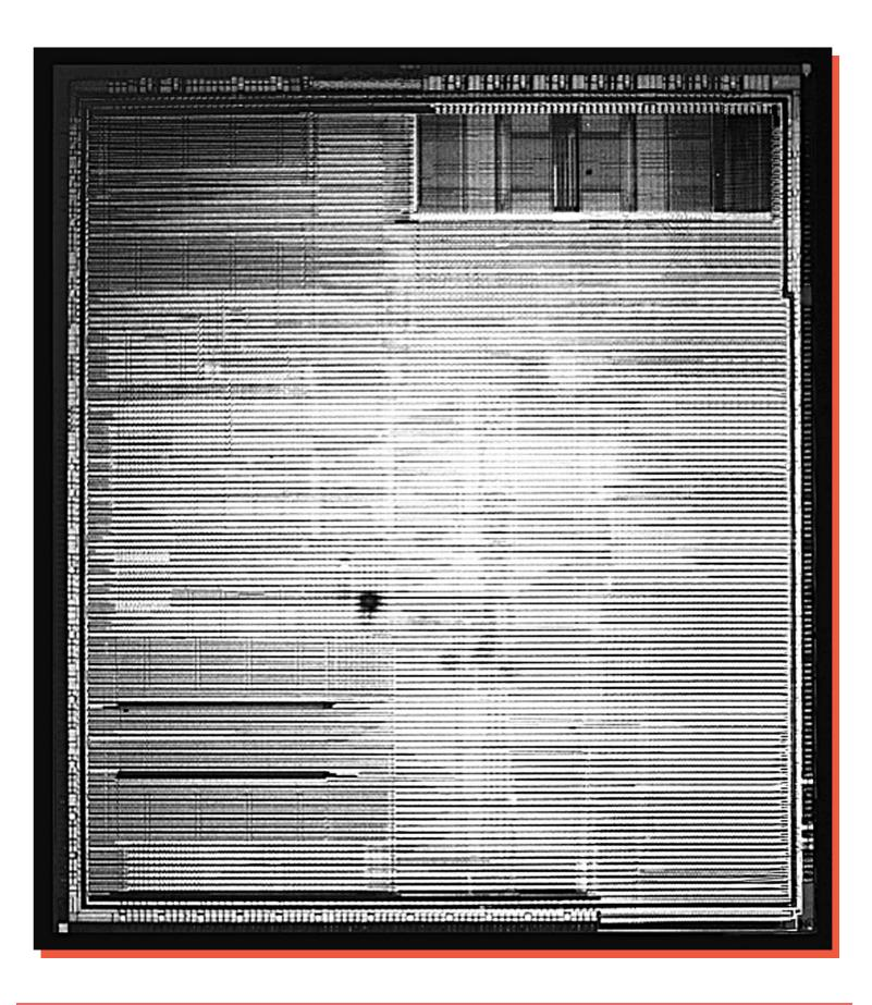
Figure 3. Whole die photograph of the Intel Pentium with MMX. Mag. 16x.
