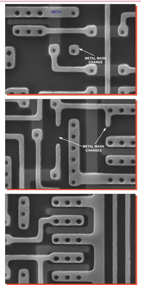
Figure 16. Topological SEM views of metal patterning. Mag. 6500x, 0°.
