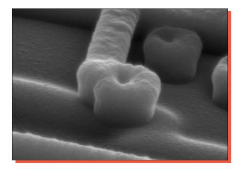
Figure 14. SEM views of overlay passivation coverage.  $60^{\circ}$ .
