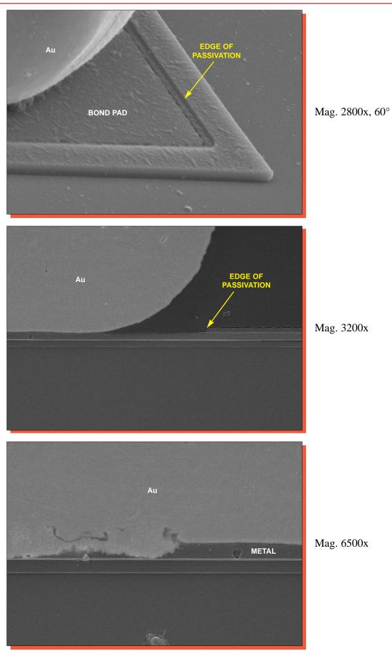
Figure 8. SEM views illustrating pad window and intermetallic formation.
