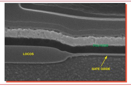
Figure 23. SEM section views of a typical birdsbeak. Mag. 52,000x.
