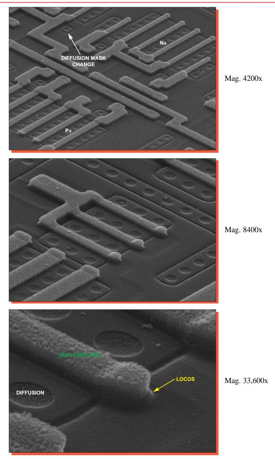
Figure 21. Perspective SEM views of polycide coverage.  $60^{\circ}$ .
