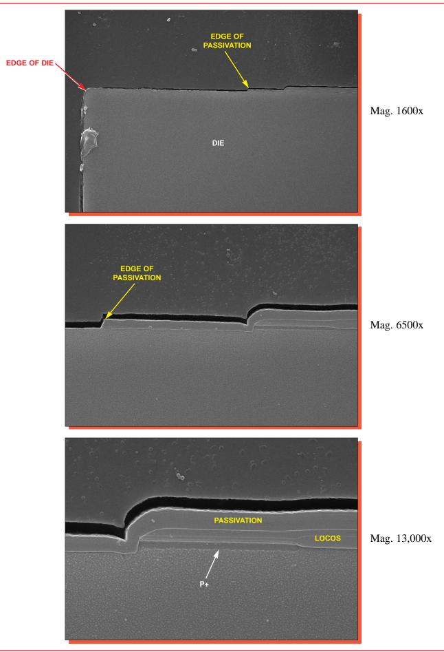
Figure 6. SEM section views of the edge seal.
