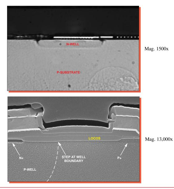
Figure 24. Section views illustrating well structure.
