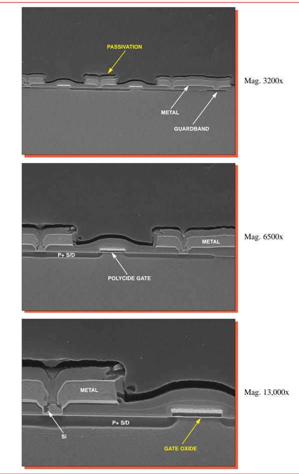
Figure 10. SEM section views of the I/O structure.
