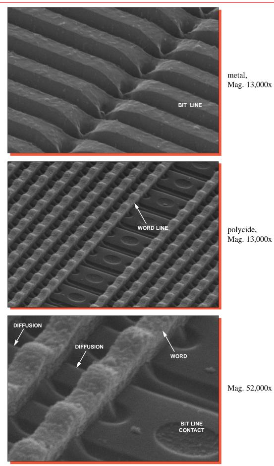
Figure 28. Detailed perspective SEM views of the NAND ROM array. 60°.
