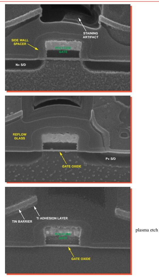
Figure 22. SEM section views of typical transistors. Mag. 52,000x.
