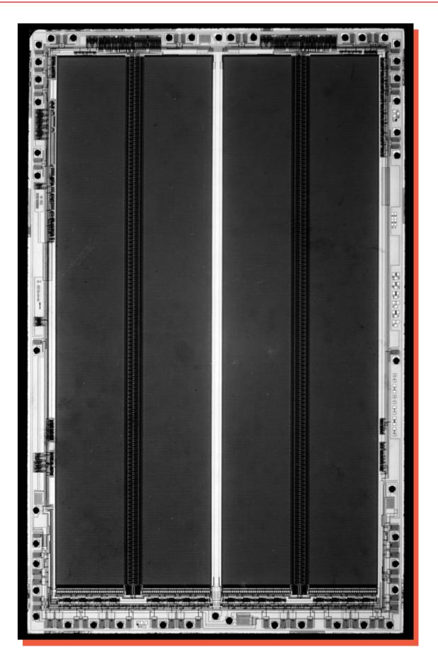
Figure 11. Whole die photograph or the NEC D23C32000A. Mag. 26x.
