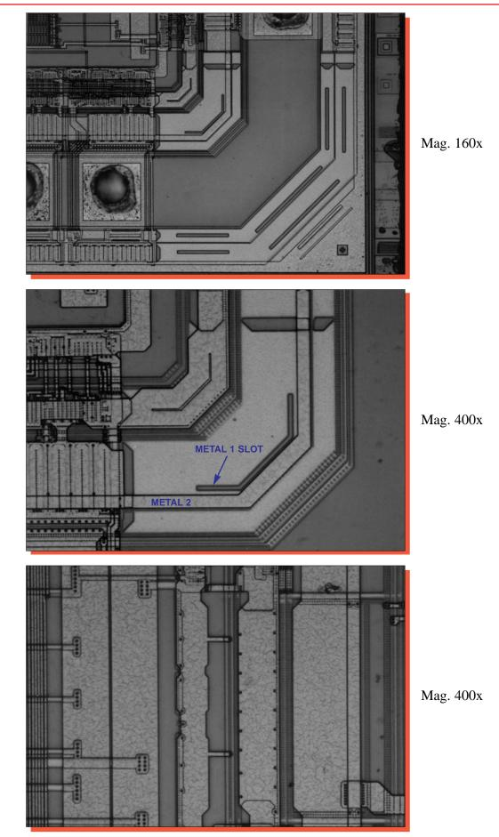
Figure 12. Optical views of slotted and beveled metal 2 bus lines.
