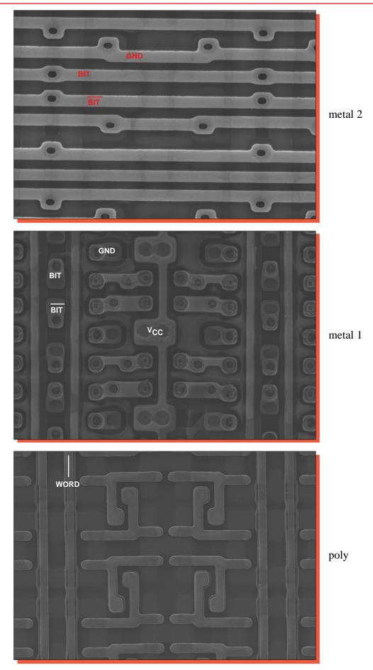
Figure 31. Topological SEM views of the SRAM cell array. Mag. 3200x.
