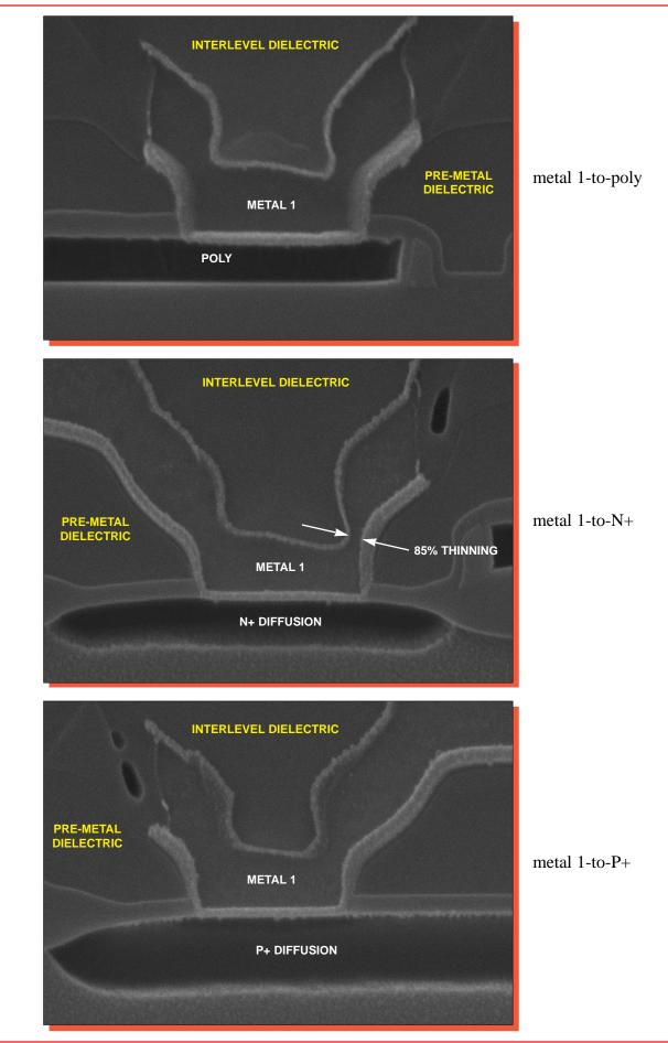
Figure 23. SEM section views of metal 1 contacts (silicon etch). Mag. 40,000x.
