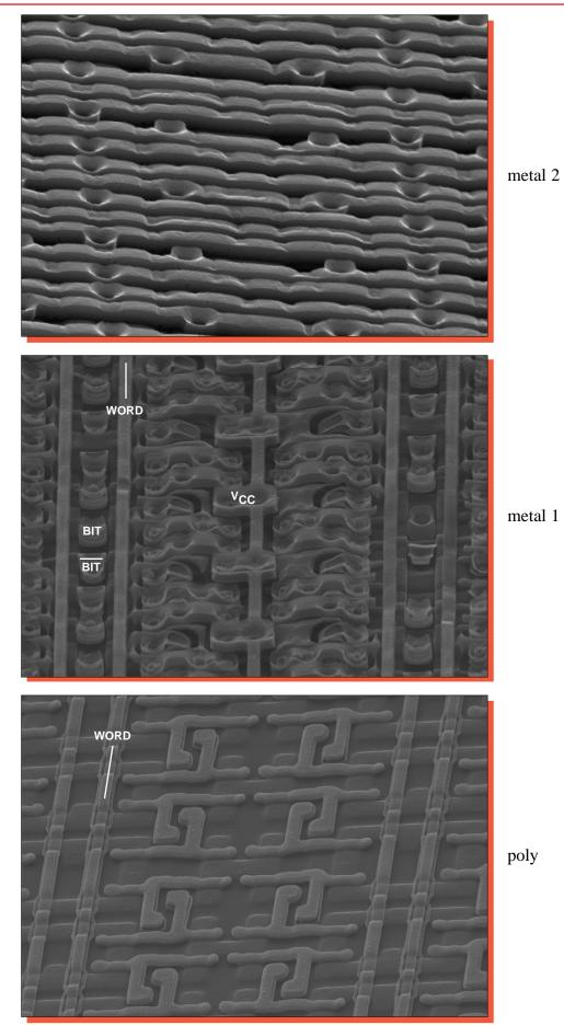
Figure 30. Perspective SEM views of SRAM cell array. Mag. 3200x, 60°.
