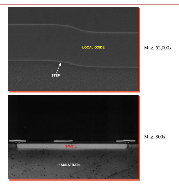
Figure 28. Section views illustrating the well structure.
