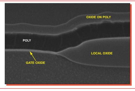
Figure 27. SEM section view of a typical local oxide birdsbeak. Mag. 52,000x.
