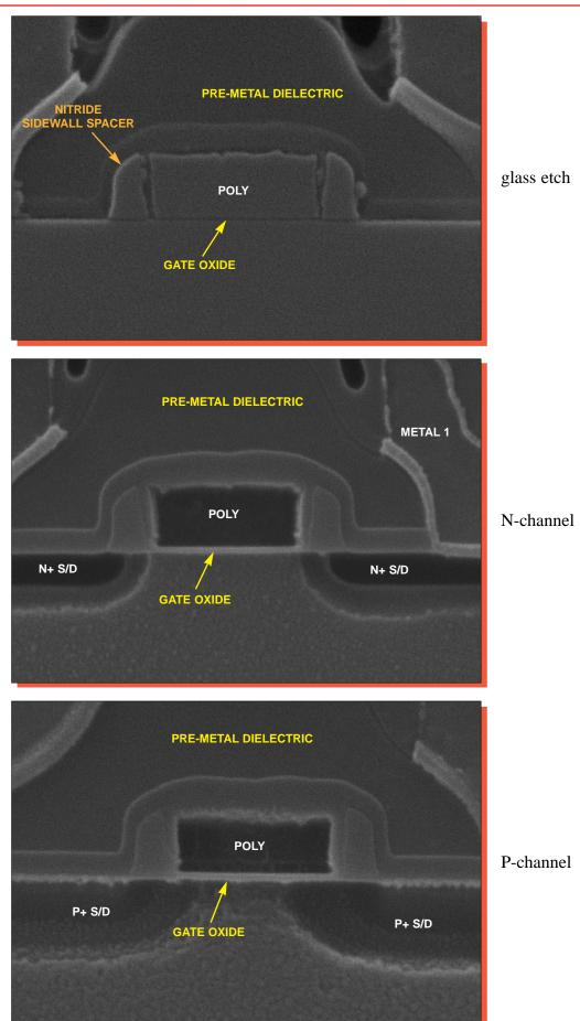
Figure 26. SEM section views of typical transistors. Mag. 52,000x.
