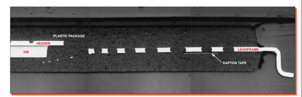
Figure 3. Optical package section view of general construction. Mag. 26x.
