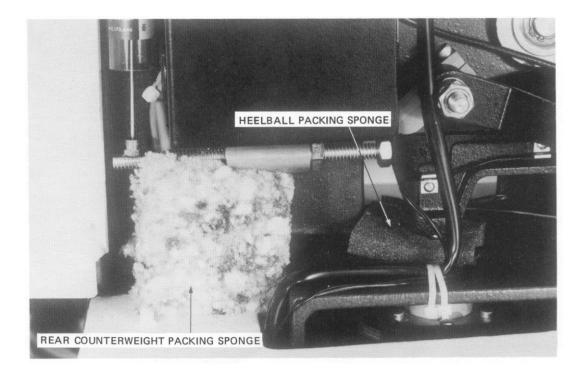
FIG. 5-3 MAIN HEAD PACKAGING - INNER LEFT SIDE
