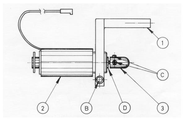
FIG. 10-8 EFO SOLENOID BRACKET ASSEMBLY (#4124-0451-0)
