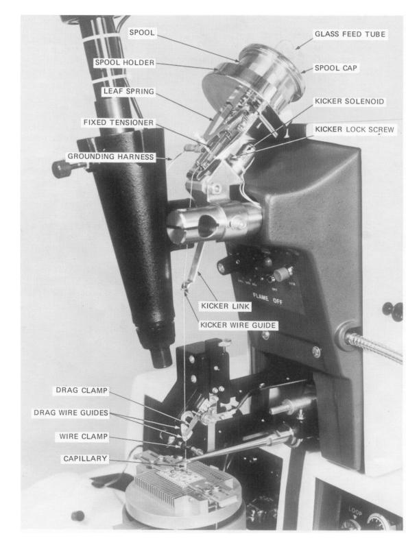
FIG. 3-12 WIRE FEED SYSTEM
