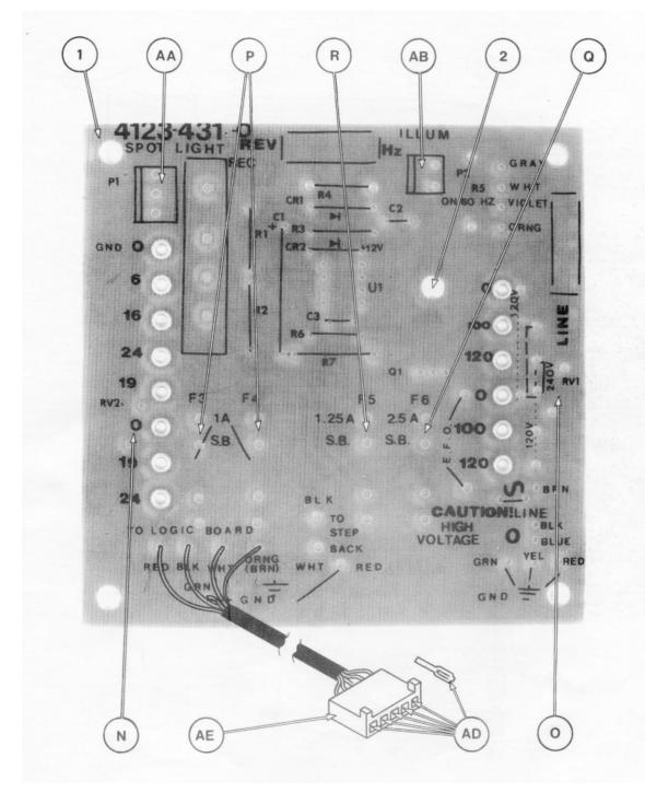
FIG 10-12 MOTHER BOARD - COMPONENTS LAYOUT (#4123-4311-0)
