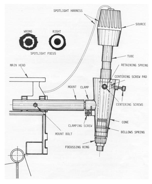
FIGURE 6-5 SPOTLIGHT MOUNTING AND ADJUSTMENT
