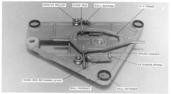
FIG. 3-5 MANIPULATOR UNDERSIDE AND X-Y FRAME
