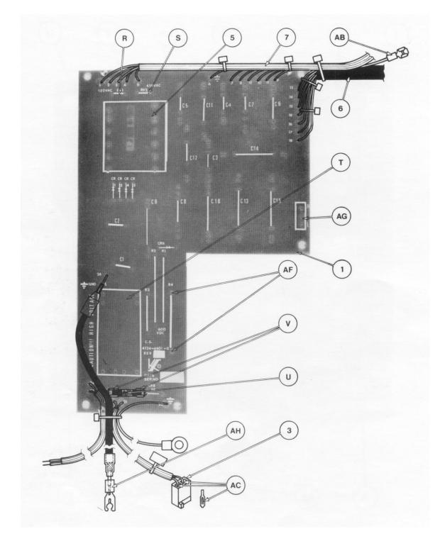
FIG. 10-13 EFO BOARD - COMPONENTS LAYOUT (#4124-4400-0)
