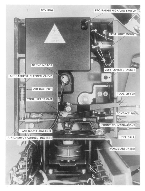
FIG. 3-9 MAIN HEAD - INNER LEFT SIDE
