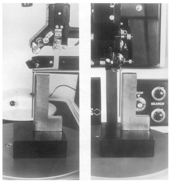
FIG. 6-1 TRANSDUCER INSERTION AND LEVELING ADJUSTMENTS
