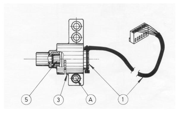
FIG. 10-8 MAIN/Z LVDT ASSEMBLY (#4123-0414-0)
