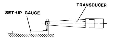
FIG. 6-3 CAPILLARY INSERTION ADJUSTMENT
