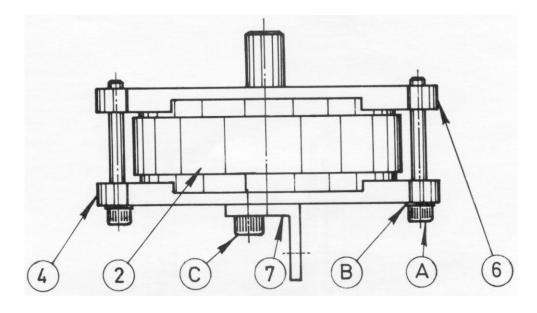
FIG. 10-4 FORCE ACTUATOR ASSEMBLY (#4123-0413-0)
