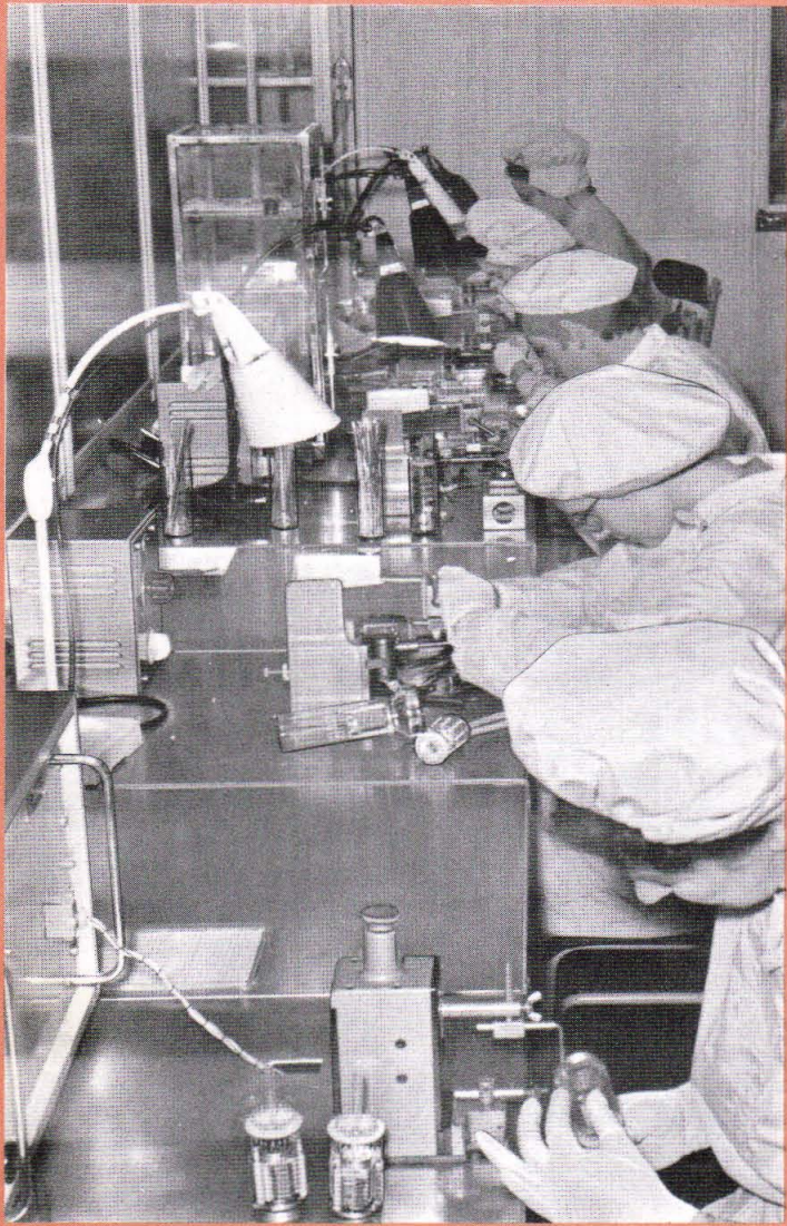
Photomultiplier tubes being assembled under clean air conditions
