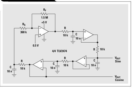
The Wien-bridge oscillator has few parts, and its frequency stability is good. Taming the distortion in a Wienbridge oscillator is harder than getting the circuit to oscillate. The quadrature oscillator only requires two op amps, but it has high distortion. Phase-shift oscillators, especially the Bubba oscillator, have less distortion coupled with good frequency stability. The improved performance of the phase-shift oscillators comes at a cost of higher component count.
