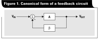
$$\frac{V_{OUT}}{V_{IN}} = \frac{A}{1 + A\beta}$$
