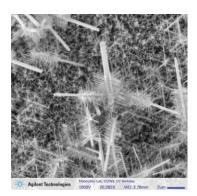
Figure 6. High resolution image of Si nanowires.
