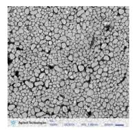
Figure 2. High resolution image of gold islands on carbon.
