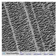
Figure 4. High resolution image of celgard.
